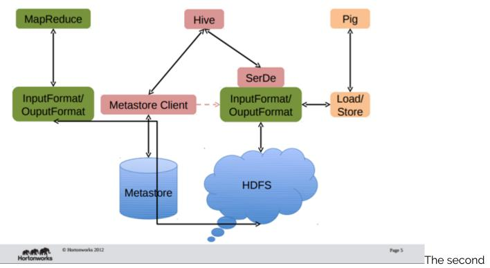
graphic shows that HCatalog exposes Hive data and metadata to MapReduce and Pig directly. This is done using the interfaces shown in yellow. The end result is that the user can work with Hive tables as if they were MapReduce key->value pairs or Pig tuples.
