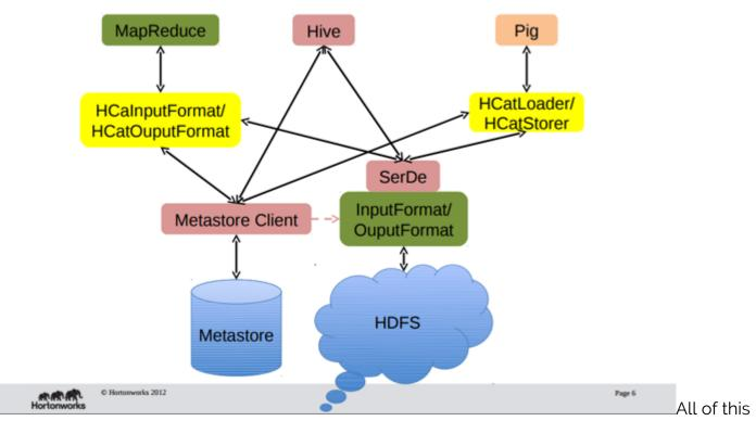
supports sharing data between programs and programmers too. For example, data can be shared with other programs as a REST web service as HCatalog exposes that. And when an Hcatalog task finishes, it can create a JMS message to signal an Apache Pig program to run.
