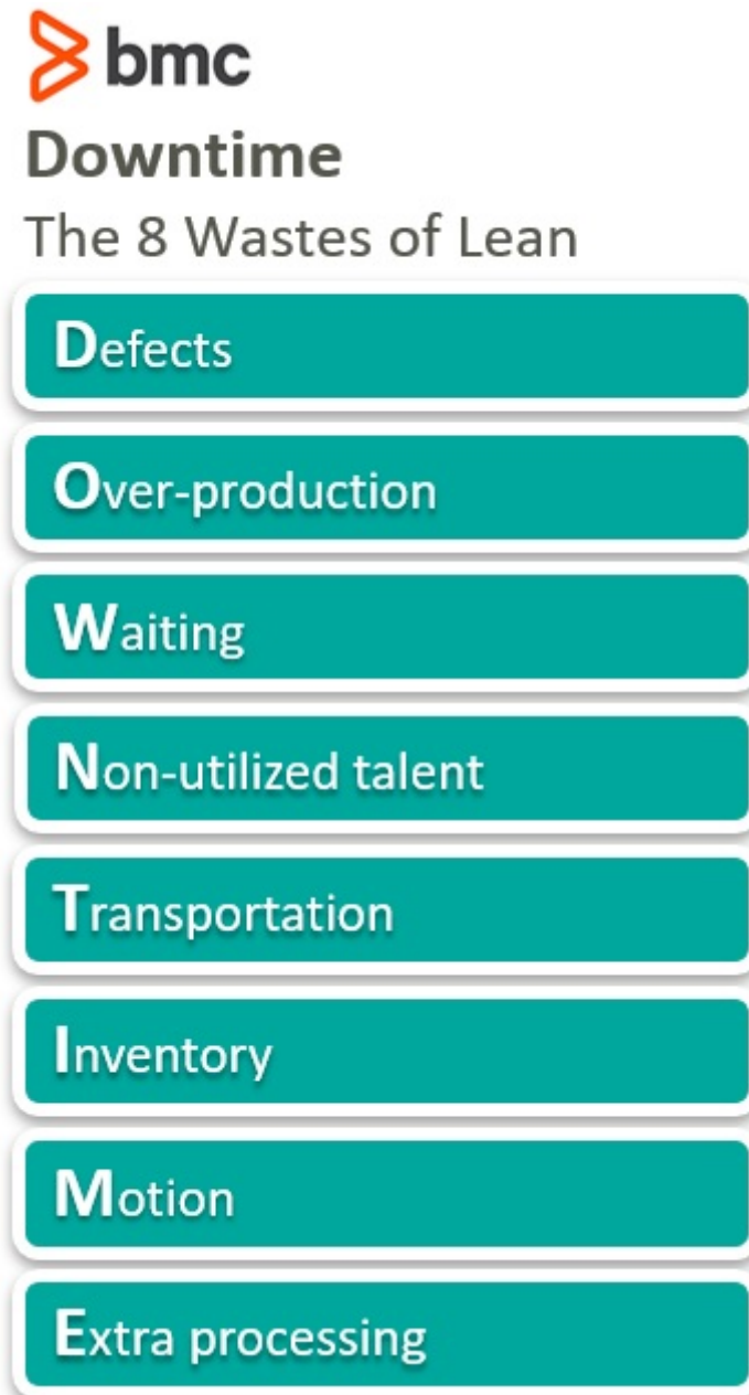
Figure 2: The eight wastes Lean aims to eliminate. The first letter of each waste category spells the acronym DOWNTIME
